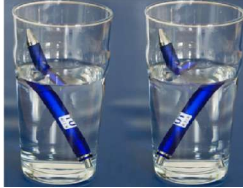
Figure 4: Refraction of light in water (left) and how light refraction might appear in a medium with a negative refractive index (right).
