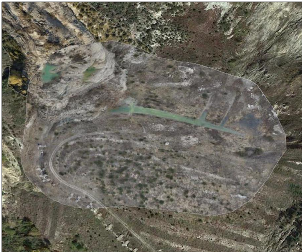
Figure 6.3 - Detailed photogrammetric orthomosaic of the investigated area. The image shows the current state of the landslide toe and the deformed drainage network. This survey area was specifically selected to evaluate morphological evolution by comparing post-event deformations with pre-2018 historical data.
